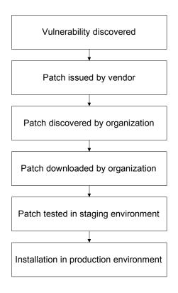
Figure 2: The patch latency stages
