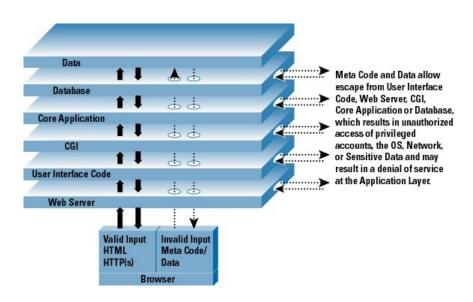
**Figure 1:** The layers of the web application
